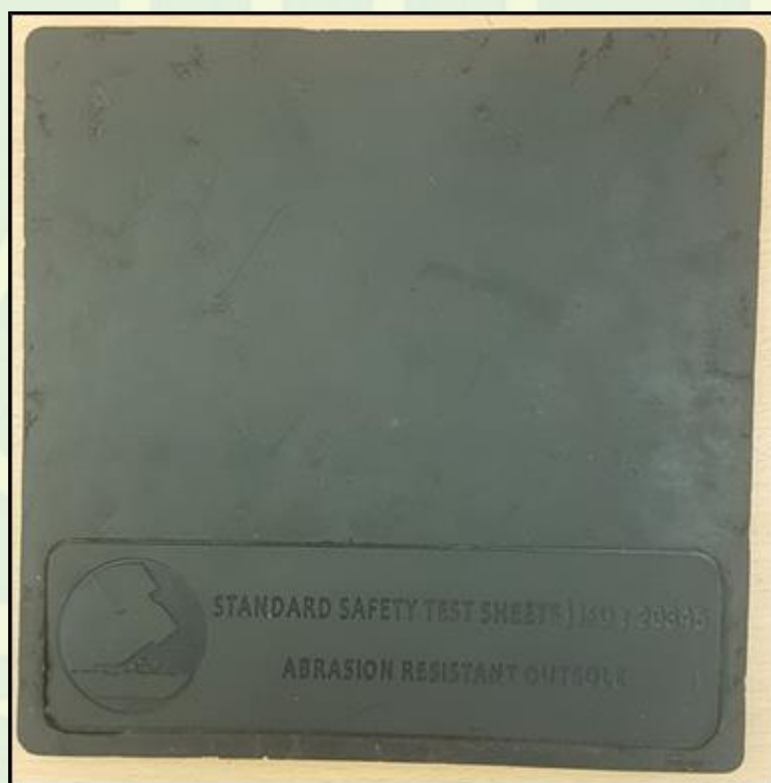
Figure 1: Photo of Rubber Slab (Nitrile Rubber Compound) for Outsole
